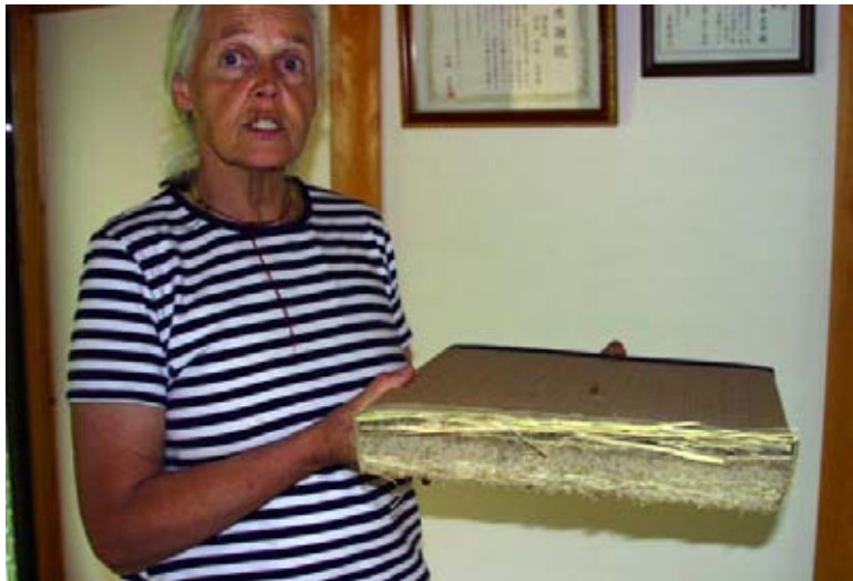
Tatami floor mats sample cross section typical of those widely used in Japan with recycling potential as wall insulation
